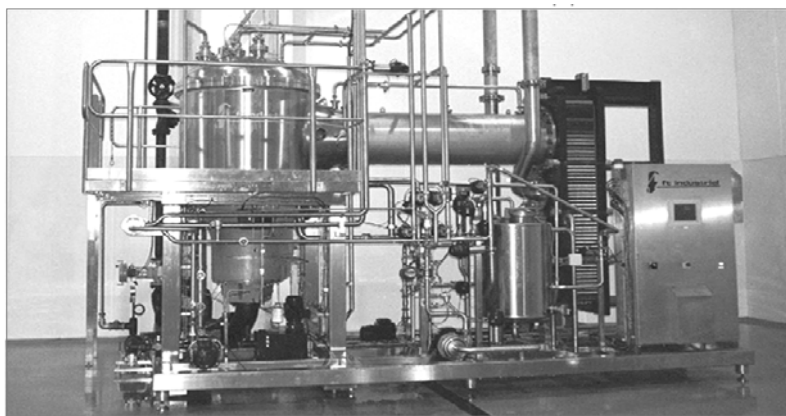
Centriterm model CT-9 installed for concentrating extracts
