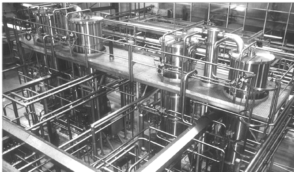
Part of installation of eight SCC 10,000 columns processing dairy products
